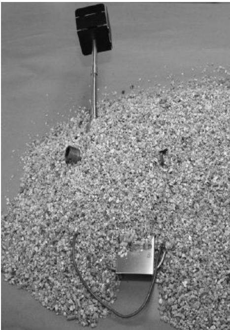
(Picture 10 – Back view) Pilot Light Assembly installed and covered with ash.
