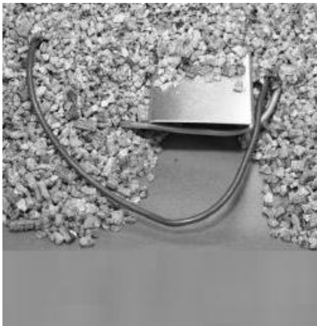
(Picture 11) Be sure to keep back of LP Air Mixer Cover clear of ash for proper air flow.
